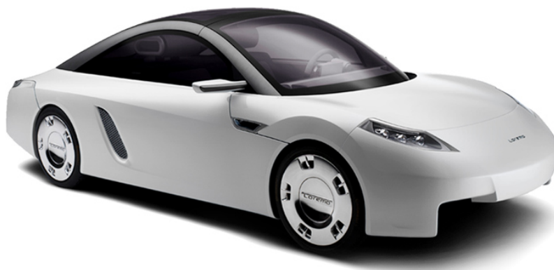
Figure 4.3 Loremo: Low resistance mobile, 450 kg, 50 g CO 2 /km, for sale in Europe in 2009
