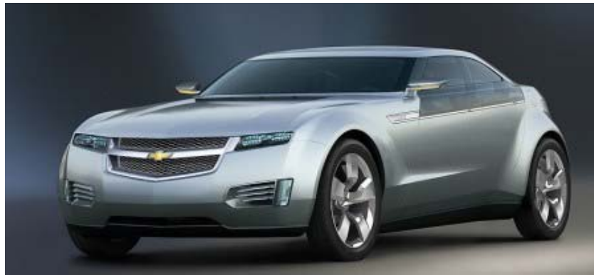
Figure 4.2 Chevrolet Volt: Plug-in hybrid, 1600 kg, 111 g CO 2 /km, on the market in 2010
